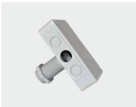
KT5 707050 5-EXITS ROOF DUCT for the wiring of photovoltaic modules, cameras or antennas. For maximum roof thickness of 60mm. Dimensions: 20 x 90 x 30mm
